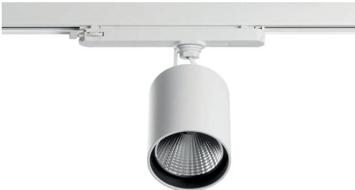
Single-piece cylindrical projector built in extruded aluminium. Different high quality Axalta paint finishes are available. The whole body of the luminaire functions as a heat sink, which allows for the integration of the system in its interior. A single-axis guidance system allows for a 355 and 90-degree inclination turn. The optical system is composed of a polycarbonate lens which casts a perfect beam without halos. LED and equipment incorporated.
