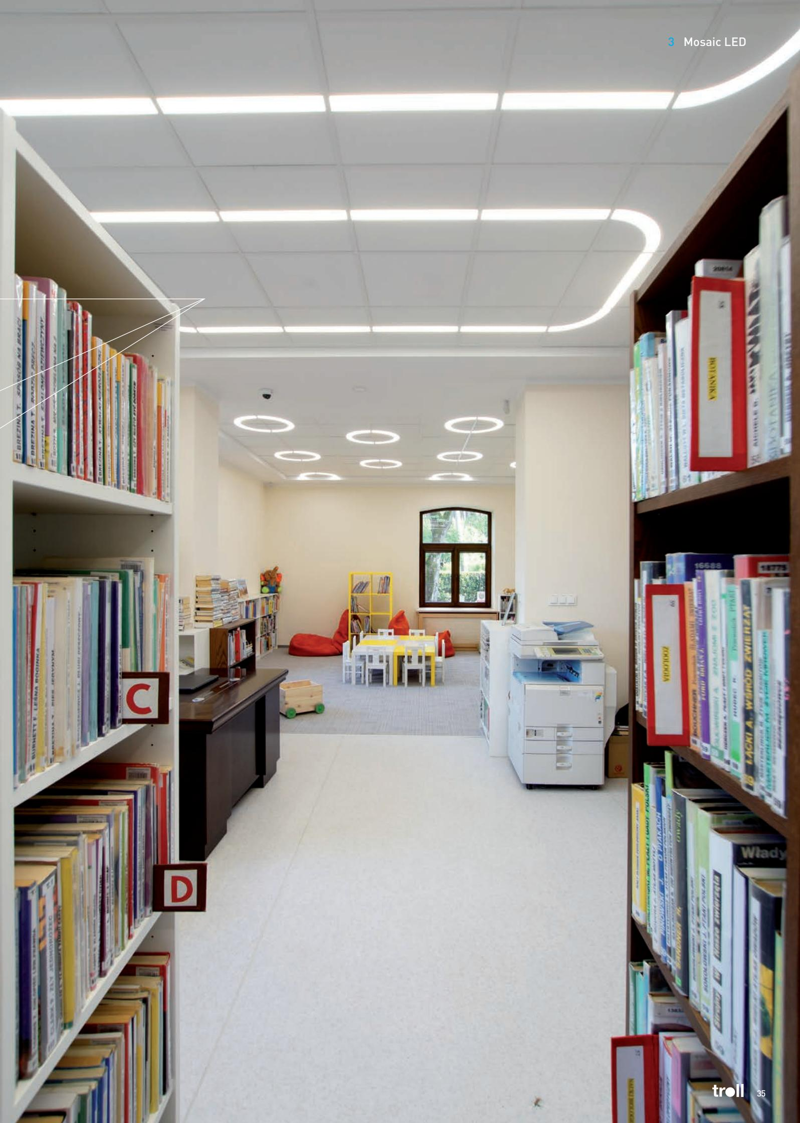
Designed system for modular ceilings based on 2 elements: a curved one and a linear. The combination of these two elements provides unlimited possibilities of lighting layouts inside. The location of the segments can be modified at any time through the specific rotation of the ceiling panels. Due to the possibility of using colour diffusers or RGB LED strips it is possible to obtain some additional colour effects. The LED system can be easily dimmed providing additional energy savings.
