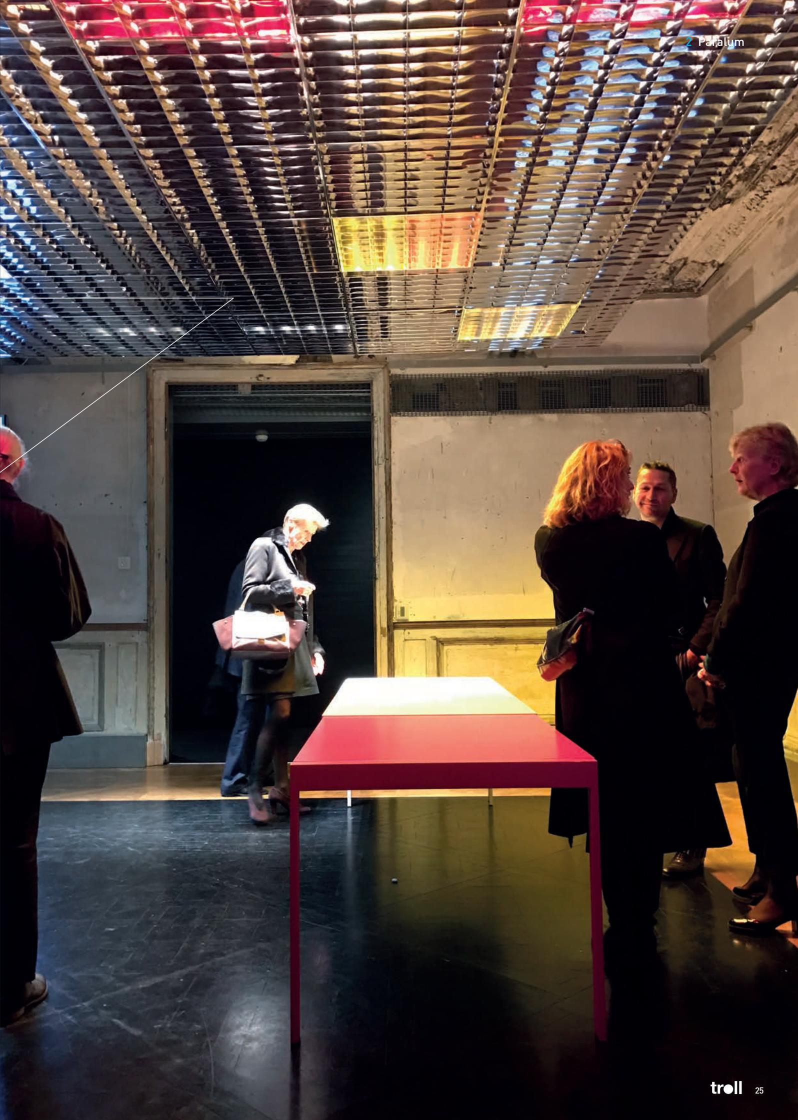
This lighting system is made up of a folding grating ceiling, which general and accent lighting modules can be placed into, as well as smoke detection, acoustics, air-conditioning and sprinkler modules, which have a built-in fire-fighting system. The French architect understands light as a building material that can create atmospheres and transmit emotions through its versatility.
